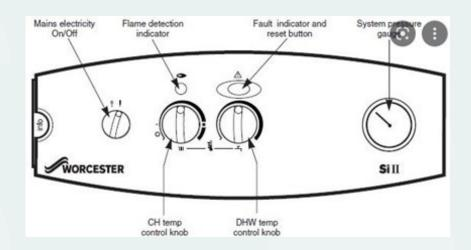
If your boiler has low water pressure, your needle on the right-hand side (see picture 1 and 2) will usually be at 0 or below 1, and the fault indication button will be flashing red.
