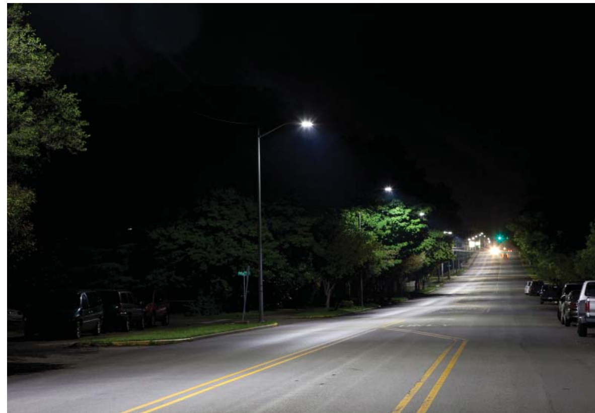
Good example of LED street lighting. The lighting equipment utilised is targeted, relatively glare free and limits the amount of light that escapes behind the fixture.
